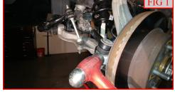
Remove the front wheels and support the lower control arm with a suitable jack.
