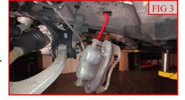
Remove the brake caliper from the knuckle. Using a suitable device, hang the caliper out of the way. DO NOT let the caliper hang by the brake line. (FIG 3)
